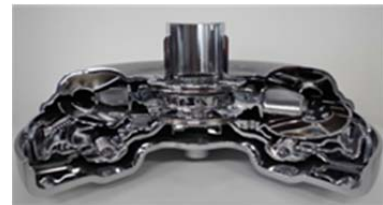
Cut section model of the Unipres Ultra Flat Torque Converter
